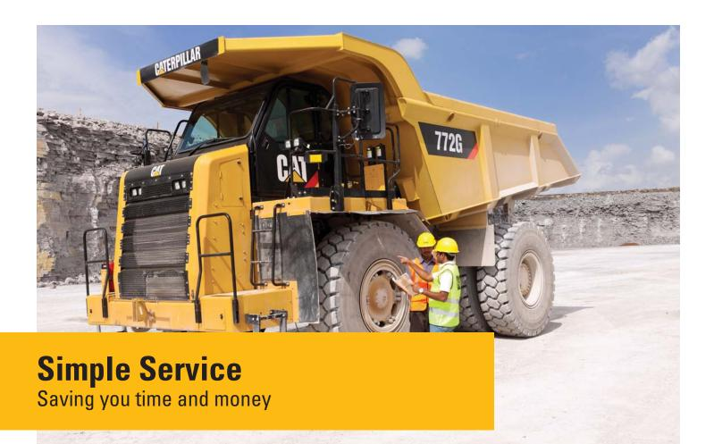
Your Cat G Series truck is designed to provide operators and technicians with easy access to common service points like engine lockout, machine system lockout, fluid level sight gauges, grease fittings, and access to the engine for regularly scheduled maintenance.
