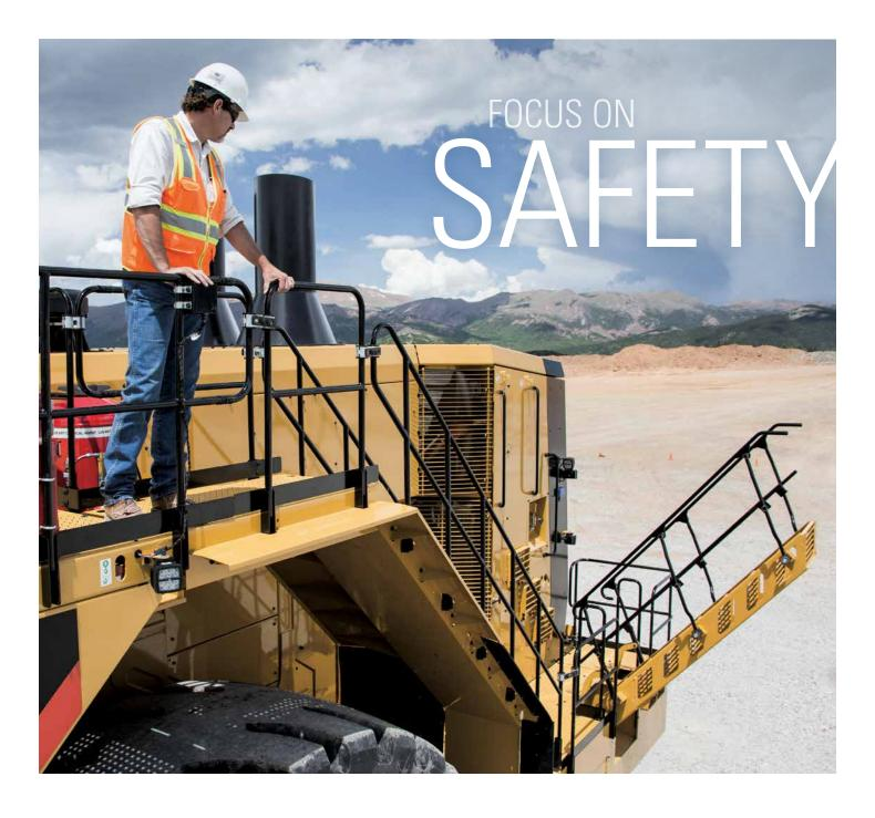
From slip-resistant surfaces and guard rails to state-of-the-art object detection technologies, the 994K is infused with features to help both operators and service personnel feel safe and confident on the job. We've improved access and egress, maximized visibility and made it possible to perform more service from the ground.
