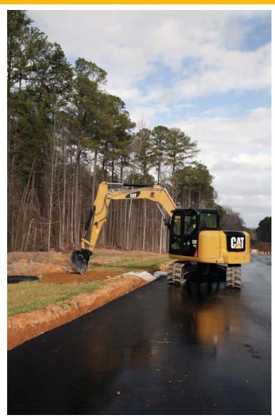
High digging forces that provide power through even the most compacted ground, coupled with direct, smooth control through responsive hydraulics, ensure that the Cat 308E2 CR SB delivers the high productivity that customers demand.
